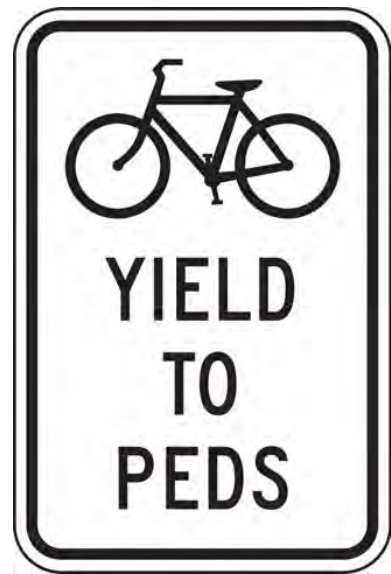
Figure 30: Signs can clarify yielding rules in shared-use environments, and may be modified based on expected user types.
