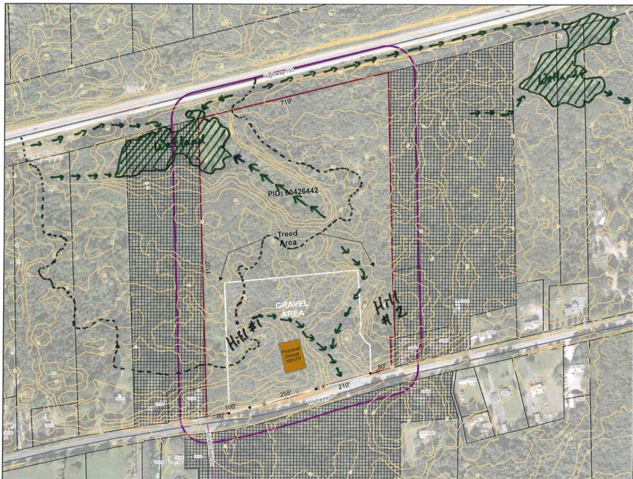
Figure 1: Watershed map of PID 60426442 and its vicinity. While the water would have naturally flowed to northward towards Hebbs Lake, a drinking water source, the water now flows to wetlands because of the raising of ground to construct Highway 103.
