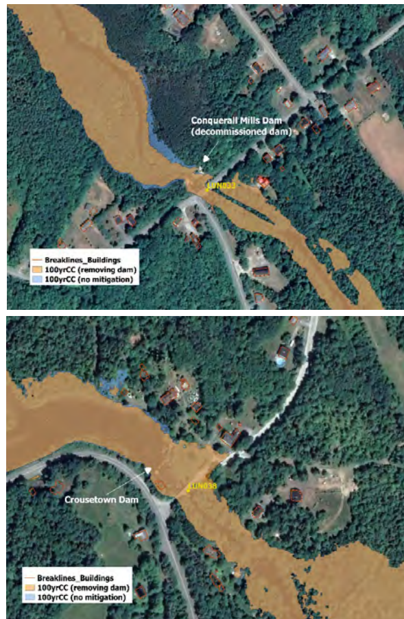
Figure 3: 100yr CC Flood Line for Conquerall Mills Dam Area and Crousetown Dam Area.
