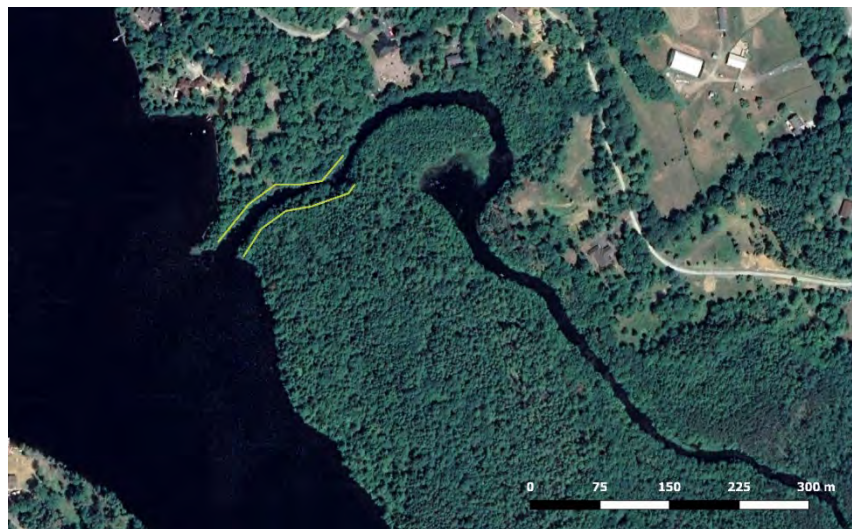
Figure 8: Approximate Location of River Banks after the Channel Widening.
